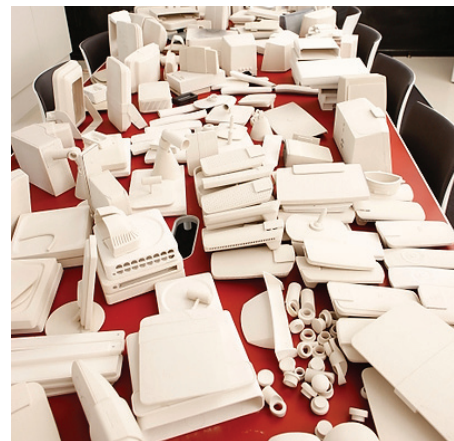
Figure 4. Using a fast and economical ZPrinter, Cisco makes prototypes frequently to evaluate design concepts.
