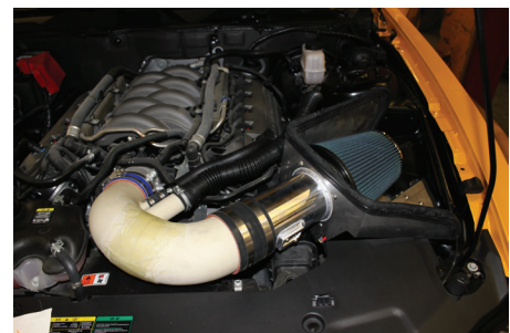
Figure 9. Example of a working prototype of a Steeda Autosports air inlet (in white) fabricated for testing with a ZPrinter.
