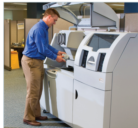
Figure 2. Z Corporation's ZPrinter 650 builds parts at the rate of 1.1 vertical inches (28 mm) per hour with length and width as large as 10 x 15 inches (254 x 381 mm).
